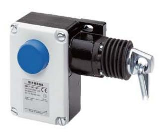
SIRIUS CABLE-OPER. SWITCH METAL HOUSING,1X M16X1.5 2NC, LATCHES ACC. EN ISO 13850 BUTTON RESET FOR CABLES UP TO TO 50M
