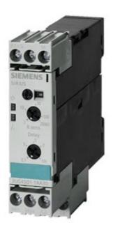
ANALOG MONITORING RELAY FILL LEVEL MONITORING RESISTANCE MONITORING FROM 2 TO 200 KOHM OVERSHOOT AND UNDERSHOOT AC/DC 24 TO 240V DC AND AC 50 TO 60 HZ 2-POINT OR 1-POINT CONTROL TRIPPING DELAYED 0.5 TO 10S 1 CHANGEOVER CONTACT SCREW TERMINAL REPLACEMENT PRODUCT F. 3UG3501
