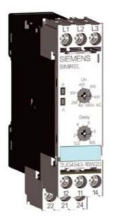
ANALOG MONITORING RELAY FILL LEVEL MONITORING RESISTANCE MONITORING FROM 2 TO 200 KOHM OVERSHOOT AND UNDERSHOOT AC/DC 24 TO 240V DC AND AC 50 TO 60 HZ 2-POINT OR 1-POINT CONTROL TRIPPING DELAYED 0.5 TO 10S 1 CHANGEOVER CONTACT SPRING-LOADED TYPE
