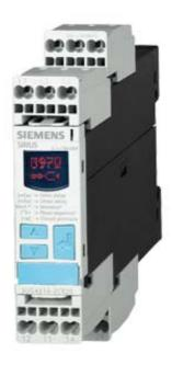
DIGITAL MONITORING RELAY UNBALANCE 0-20% REVERSIBLE PHASE SEQUENCE PHASE FAILURE 3X 160 TO 690V AC 50 TO 60 HZ UNDERVOLTAGE 160-690V HYSTERESIS 1-20V ON AND OFF DELAY 0-20S 2 CHANGEOVER CONTACTS SPRING LOADED CONNECTION
