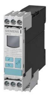
DIGITAL MONITORING RELAY FOR THREE-PHASE LINE VOLTAGE REVERSIBLE PHASE SEQUENCE PHASE FAILURE 3X 160 TO 690V AC 50 TO 60 HZ UNDERVOLT. AND OVERVOLT. 160-690V HYSTERESIS 1-20V 0-20S EACH FOR UMIN AND UMAX 1 W FOR UMIN 1W FOR UMAX SCREW TERMINAL REPLACEMENT PRODUCT F. 3UG3041-1BP50
