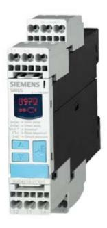
DIGITAL MONITORING RELAY FOR THREE-PHASE LINE VOLTAGE REVERSIBLE PHASE SEQUENCE PHASE FAILURE 3X 160 TO 690V AC 50 TO 60 HZ UNDERVOLT. AND OVERVOLT. 160-690V HYSTERESIS 1-20V 0-20S EACH FOR UMIN AND UMAX 1 W FOR UMIN 1W FOR UMAX SPRING-LOADED TYPE
