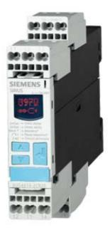
DIGITAL MONITORING RELAY FOR 3-PHASE LINE VOLT. W. N COND. REVERSIBLE PHASE SEQUENCE PHASE FAILURE 3X 160 TO 690V AC 50 TO 60 HZ UNDERVOLT. AND OVERVOLT. 160-690V HYSTERESIS 1-20V 0-20S EACH FOR UMIN AND UMAX 1 W FOR UMIN 1 W FOR UMAX SPRING-LOADED TERMINAL
