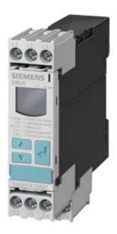
DIGITAL MONITORING RELAY FOR THREE-PHASE LINE VOLTAGE AUT. CORRECTION OF PHASE SEQUENCE PHASE FAILURE 3X 160 TO 690V AC 50 TO 60 HZ UNDERVOLT. AND OVERVOLT. 160-690V HYSTERESIS 1 -20V OFF DELAY 0-20S 1 W FOR POWER SYSTEM FAULTS 1W FOR PHASE CORRECTION SCREW TERMINAL
