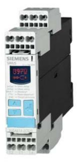
DIGITAL MONITORING RELAY FOR THREE-PHASE LINE VOLTAGE AUT. CORRECTION OF PHASE SEQUENCE PHASE FAILURE 3X 160 TO 690V AC 50 TO 60 HZ UNDERVOLT. AND OVERVOLT. 160-690V HYSTERESIS 1 -20V OFF DELAY 0-20S 1 W FOR POWER SYSTEM FAULTS 1W FOR PHASE CORRECTION SPRING-LOADED TYPE
