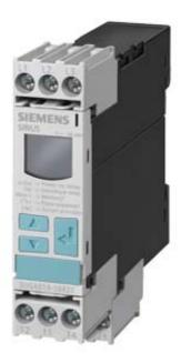
DIGITAL MONITORING RELAY FOR THREE-PH. VOLT. W. N COND. AUT. CORRECTION OF PHASE SEQUENCE PHASE FAILURE 3X 160 TO 690V AC 50 TO 60 HZ UNDERVOLT. AND OVERVOLT. 160-690V HYSTERESIS 1 -20V OFF DELAY 0-20S 1 W FOR POWER SYSTEM FAULTS 1W FOR PHASE CORRECTION SCREW TERMINAL
