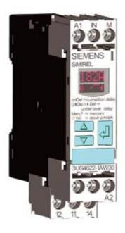
DIGITAL MONITORING RELAY CURRENT MONITORING, 22.5MM FROM 2 TO 500MA AC/DC OVERSHOOT A. UNDERSHOOT AC/DC 24 TO 240V DC AND AC 50 TO 60 HZ ON AND SPIKE DELAY 0.1 TO 20S HYSTERESIS 0.1 TO 250MA 1 CO CONTACT W. OR W/O ERROR MEMORY SCREW CONNECTION REPLACEMENT PRODUCT FOR 3UG3521-1AL20,
