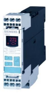
DIGITAL MONITORING RELAY CURRENT MONITORING, 22.5MM FROM 2 TO 500MA AC/DC OVERSHOOT AND UNDERSHOOT SUPPLY VOLTAGE: AC/DC 24V DC AND AC 50 TO 60 HZ NO GALVANIC ISOLATION FROM MEASURING CIRCUIT STARTUP AND INTERF. PEAK DELAY 0.1 TO 20S HYSTERESIS 0.1 TO 250MA 1 CO CONTACT W. OR W/O ERROR LOG AUTOM. RESET SPRING-LOADED CONNECTION
