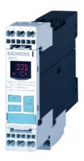
DIGITAL MONITORING RELAY CURRENT MONITORING, 22.5MM FROM 0.05 TO 10A AC/DC OVERSHOOT AND UNDERSHOOT AC/DC 24 TO 240V DC AND AC 50 TO 60 HZ STARTUP AND INTERF. PEAK DELAY 0.1 TO 20S HYSTERESIS 0.01 TO 5A 1 CHANGEOVER CONTACT W. OR W/O ERROR LOG SPRING-LOADED TYPE
