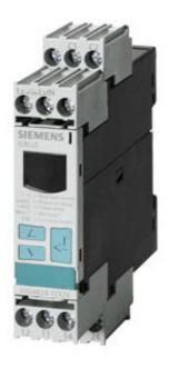
DIGITAL MONITORING RELAY FOR FAULT CURRENT MONITORING (W. CO CONTACT 3UL22) SETTING RANGE 10 TO 100% OF CO CONTACT NOM. VALUE SEPARATE FOR ALARM THRESHOLD AND SWITCH-OFF VALUE AC 90 TO 690V AC 50 TO 60 HZ STARTUP AND TRIPPING DELAYED 0.1 TO 20S SWITCH-OFF HYSTERESIS TO 50% ALARM HYSTERESIS 5% FIXED 2 CHANGEOVER CONTACTS W. OR W/O ERROR LOG SCREW TERMINAL REPLACEMENT PRODUCT F. 3UL21
