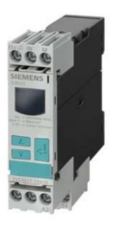
DIGITAL MONITORING RELAY VOLTAGE MONITORING, 22.5MM FROM 0.1 TO 60V AC/DC OVERSHOOT AND UNDERSHOOT SUPPLY VOLTAGE: AC/DC 24V DC AND AC 50 TO 60 HZ NO GALVANIC ISOLATION FROM MEASURING CIRCUIT INTERF. PEAK DELAY 0.1 TO 20S HYSTERESIS 0.01 TO 30V 1 CO CONTACT W. OR W/O ERROR LOG SCREW TERMINAL REPLACEMENT PRODUCT FOR 3UG3531-1AC..
