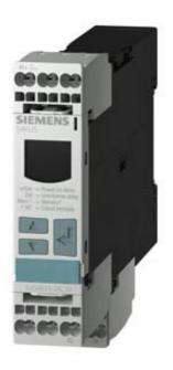
DIGITAL MONITORING RELAY VOLTAGE MONITORING, 22.5MM FROM 17 TO 275V AC/DC OVERSHOOT AND UNDERSHOOT INTERNAL POWER SUPPLY DC AND AC 50 TO 60 HZ SPIKE DELAY 0.1 TO 20S HYSTERESIS 0.1 TO 150V 1 CHANGEOVER CONTACT SPRING-LOADED TYPE
