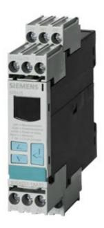
DIGITAL MONITORING RELAY SPEED MONITORING FROM 0.1 TO 2200 REV/MIN OVERSHOOT AND UNDERSHOOT SUPPLY VOLTAGE: AC/DC 24V DC AND AC 50 TO 60 HZ NO GALVANIC ISOLATION FROM MEASURING CIRCUIT STARTUP DELAY 1 TO 900S TRIP DELAY 0.1 TO 99.9S HYSTERESIS 0.1 TO 99 REV/MIN 1 CO CONTACT W. OR W/O ERROR LOG SCREW TERMINAL REPLACEMENT PRODUCT FOR 3UG3051
