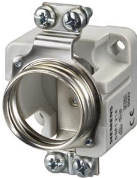
DIAZED-BASE DIII 63A AC690V DC500V SADDLE/SADDLE TERMINAL SCREW TYPE
