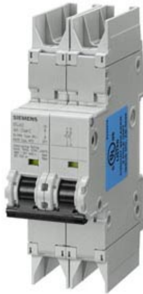
CIRCUIT BREAKER 10KA, 2POLE, C, 20A ACC. TO UL 489 - 480Y/277V
