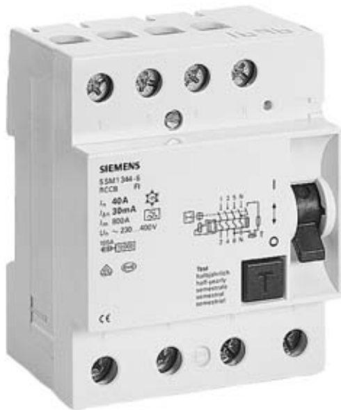
RES.CURRENT OP.CIRCUIT BREAKER TYPE A PSE/SSF D=55MM 40A 3+N-POL IFN 30MA 400V 4MW 50-400HZ
