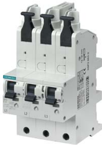
MAIN CONDUCTOR CIRCUIT-BREAKER (SHU),3X1-POLE,E 20 A,230/400 V FOR MOUNTING ONTO 40MM BUSBAR
