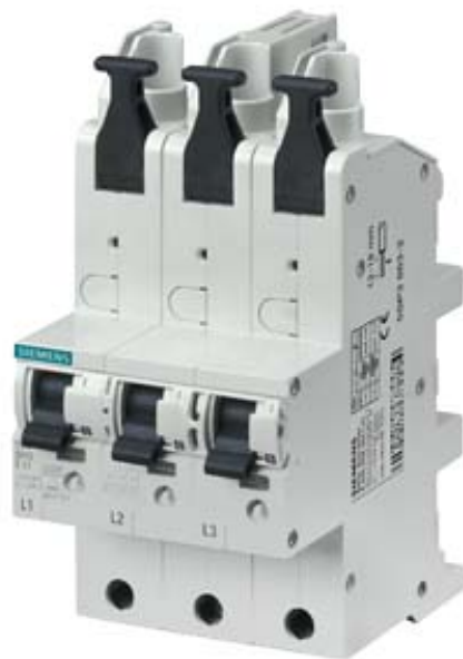
MAIN CONDUCTOR CIRCUIT-BREAKER (SHU),3X1-POLE,E 40 A,230/400 V FOR MOUNTING ONTO 40MM BUSBAR
