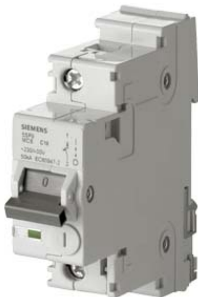
CIRCUIT BREAKER 230/400V 50KA ACC. IEC 947-2, T92 1-POLE, C, 40A
