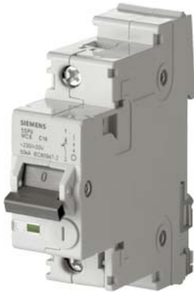
CIRCUIT BREAKER 230/400V 50KA ACC. IEC 947-2, T92 1-POLE, C, 63A
