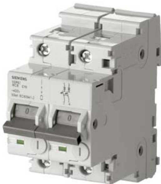
CIRCUIT BREAKER 400V 50KA ACC. IEC 947-2, T92 2-POLE, C, 50A
