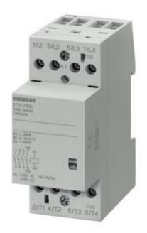
INSTA CONTACTOR W. 3 NO CONT. AND 1 NC CONTACT CONTACT FOR 230, 400 V AC 24 A ACTIVATION 230 V AC 220 V DC
