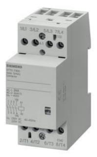
INSTA CONTACTOR W. 2 NO CONT. AND 2 NC CONTACT CONTACT FOR 230, 400 V AC 24 A ACTIVATION 230 V AC 220 V DC
