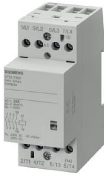
INSTA CONTACTOR W. 2 NO CONT. AND 2 NC CONTACT CONTACT FOR 230, 400 V AC 24 A ACTIVATION 24 V AC/DC
