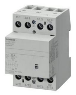
INSTA CONTACTOR W. 2 NO CONT. AND 2 NC CONTACTS CONTACT FOR 230, 400 V AC 40 A ACTIVATION 230 V AC 220 V DC
