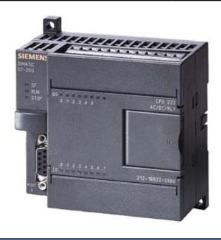
SIMATIC S7-200, CPU 222 COMPACT UNIT, AC POWER SUPPLY 8 DI DC/6 DO RELAY 4 KB CODE/2 KB DATA, PROFIBUS DP EXTENDABLE
